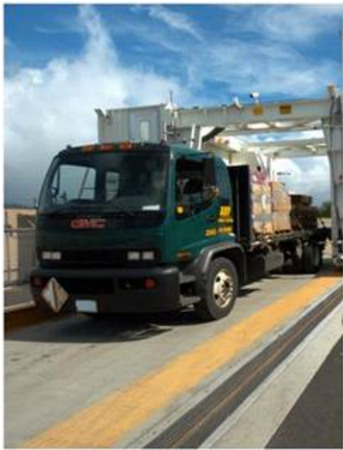
Figure 4. Fixed vehicle X-ray inspection system ( www.defence.gov )
